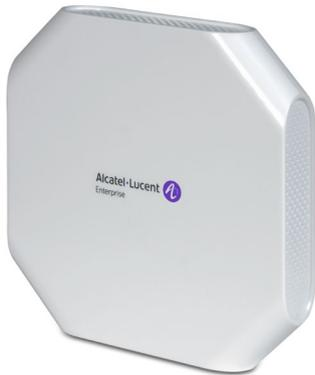
OmniAccess AP1101 is a dual-radio, 802.11ac 2x2 MIMO, indoor wireless access point. Powered by multi-core CPU processor, the OmniAccess AP1101 has fast encoding and decoding capabilities and provides reliable multiuser access. It supports up to 1.2Gb/s wireless data rate and up to 64 simultaneous clients association.
